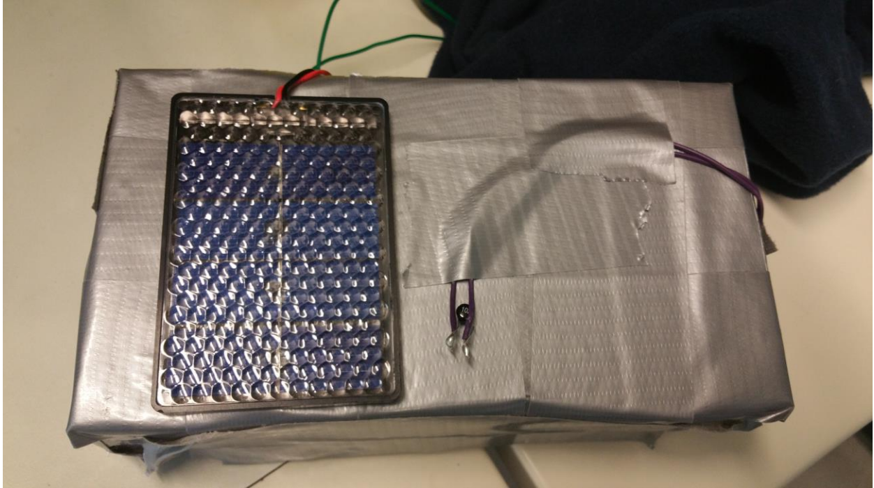
Picture 4: Solar Cell (left) and Thermistor (right) on reverse side of payload
